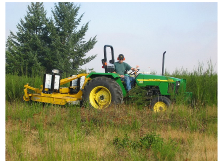
Wet blade mower in action at McChord Air Force Base.
